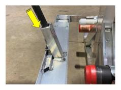
ii. (1) Pull DOWN the lift bar, (2) PLACE support bar between side of rack base and wheel dolly. Make sure to center on both sides.
