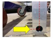
iv. Insert and run wheel dolly rack axle through rack tube, insert lynch pins on EACH side of axle. Close lynch pins on each side.
